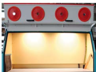
Blasting room with front flap Grating, Interior lighting, Blasting nozzle and air blow out gun
