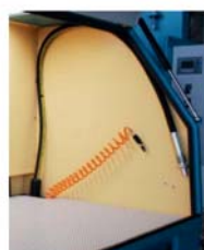
Blasting room with front flap Grating, Interior lighting, Blasting nozzle and air blow out gun
