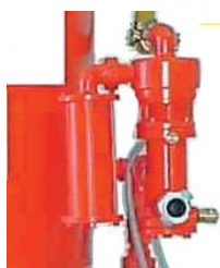
Kesselentlüftung Tank de-pressuring device
